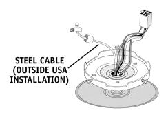
**Step 4.** Hold the switch housing close to the fan and connect the motor plug to the switch housing socket. The connectors are keyed to ensure correct alignment during installation - *Do not force!*
